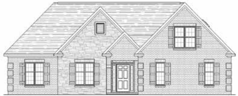
ELEV. A SHOWN W/ OPT. BONUS RM, OPT. BRICK-STONE-BRICK & OPT. QUOIN CORNERS
