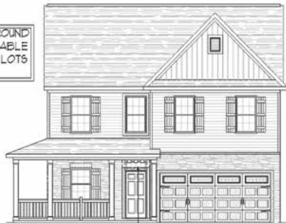
OPT. TRANSOM ELEV. A SHOWN W/ OPT. 9' CLG, OPT. BOARD & BATTEN, OPT. STONE, OPT. WRAP-AROUND PORCH, OPT. RAILING & OPT. PLANK SHUTTERS
