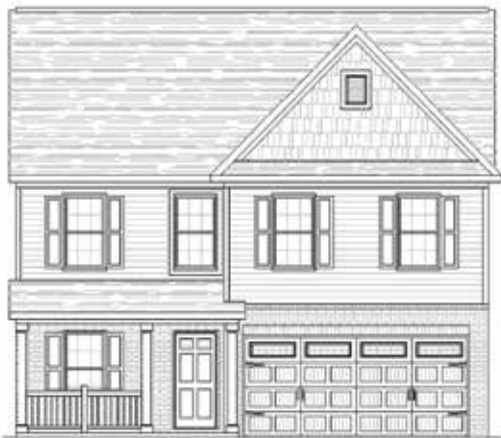
ELEV. A SHOWN W/ OPT. SHAKE, OPT. BRICK, OPT. FULL PORCH & OPT. RAILING
