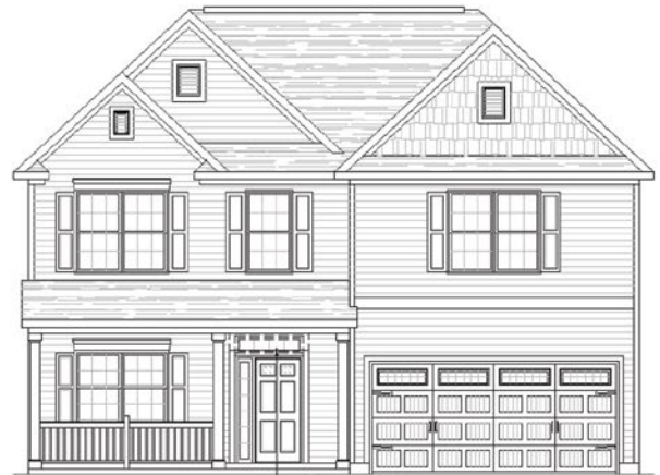
OPT. TRANSOM ELEV. B SHOWN W/ OPT. 9' CLG, OPT. HIP ROOF, OPT. FULL PORCH, OPT. RAILING, OPT. SIDE LT, OPT. BOARD & BATTEN #1 & OPT. CROSSHEADS
