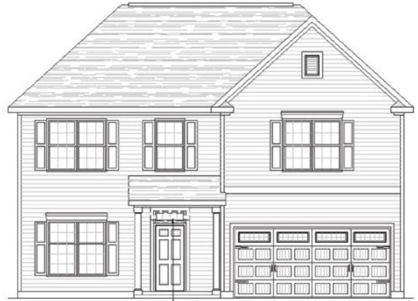
OPT. TRANSOM ELEV. A SHOWN W/ OPT. 9' CLG, OPT. HIP ROOF & OPT. CROSSHEADS
