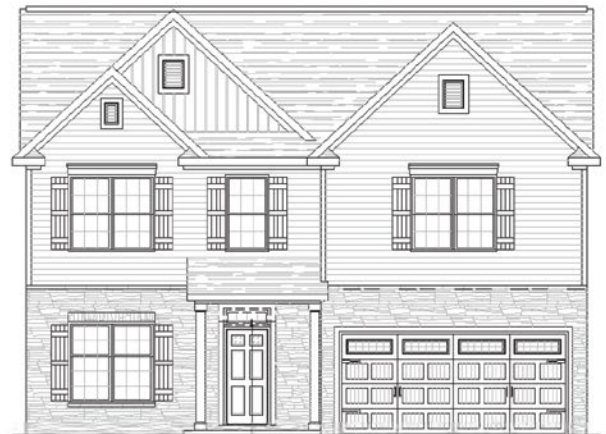
OPT. TRANSOM ELEV. B SHOWN W/ OPT. STONE, OPT. 9' CLG, OPT. BOARD & BATTEN #2 & OPT. CROSSHEADS
