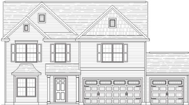
ELEV. B SHOWN W/ OPT. 3 CAR GARAGE, OPT. BAY, OPT. SHAKE #1 & OPT. CROSSHEAD
