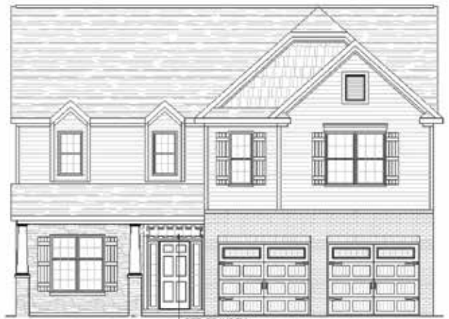
ELEV. A SHOWN W/ OPT. 9' CLG, OPT. STONE & BRICK, OPT. SHAKES & OPT. STONE COLS
